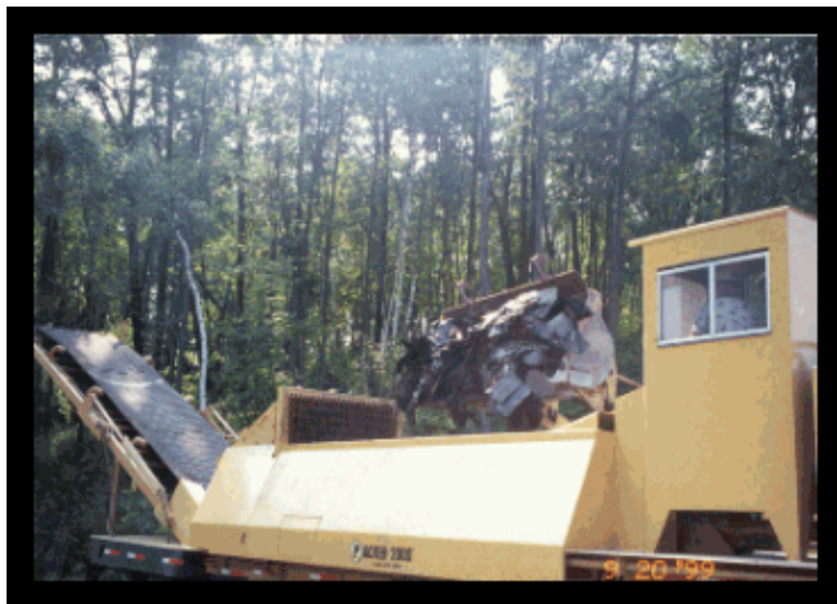
Packer Industries demonstrating their rotary drum grinder on collected asphalt shingles at A. Marcellino
