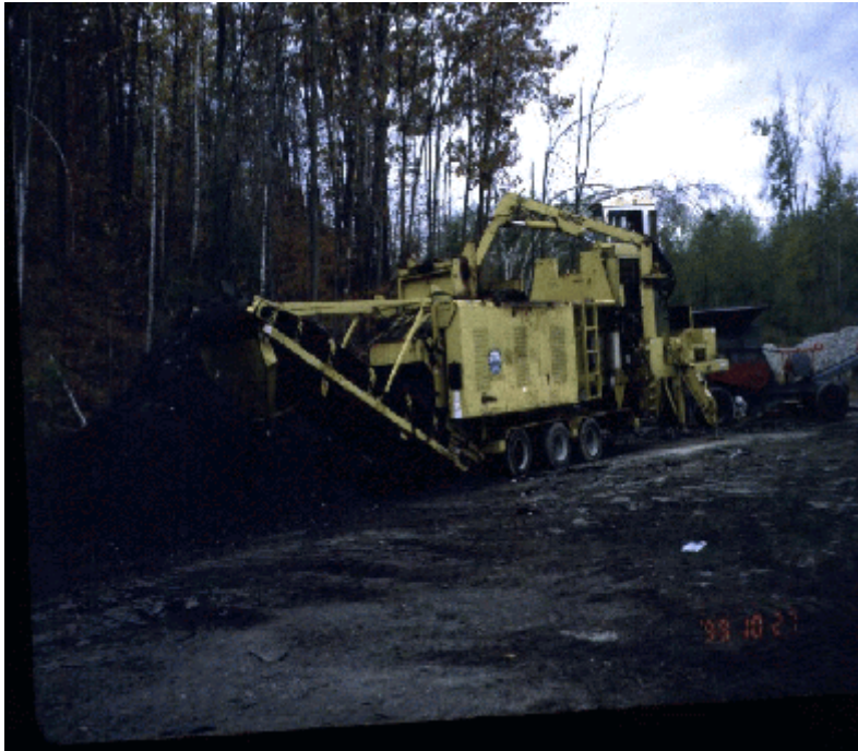
Chittenden Solid Waste District's grinder processing some of the 394 tons of waste asphalt shingles collected from April 1999 to July 2000.
